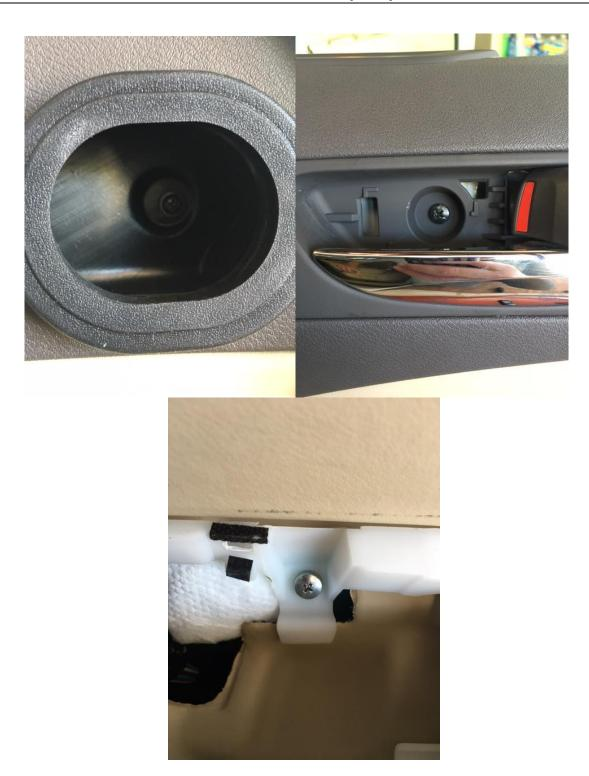
3.5 Once the five phillips screw are removed, use your panel tool (or your hands) to pry the door panel away from the door, starting at the bottom and working your way up the sides, finishing at the top.
